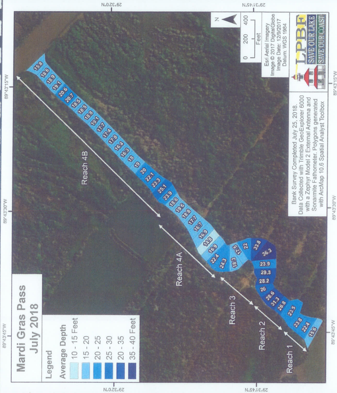
Figure 8: Polygons used to summarize the average depths (feet) of the Mardi Gras Pass in Reaches 1 through 4A. Average depth statistics computed using raw bathymetry points
